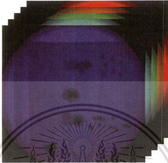
Figure 2.3 Three dimensional multispectral image cube consists of two spatial dimension and one spectral dimension.
