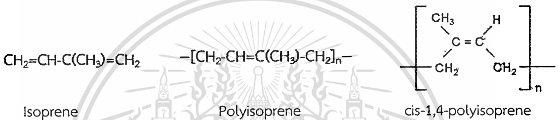
Figure 2.2 Chemical structure of natural rubber latex (cis-1,4-polyisoprene).
