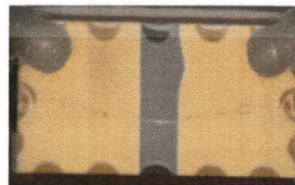
Fig. 7 Microphotograph of the damaged PZT element due to a crack across from left to right.
