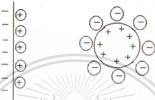
Figure 5.9: Charge distribution during cathodic codeposition [40].
