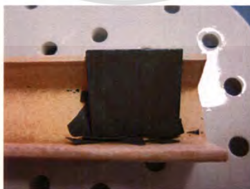
Figure 4.22: Physical characteristics of MnCo 2 O 4 -PVD coated on FeCoNi alloy after oxidation at 800 °C in O 2 -5%H 2 O at a total flow rate of 10 L/h for 500 h.
