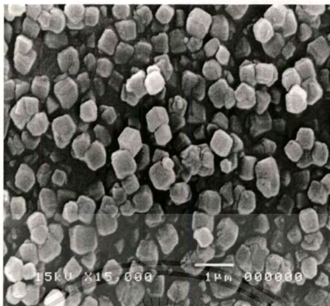
Figure 4.8 (Continued) Scanning electron micrograph of zeolite A with different basicity.
