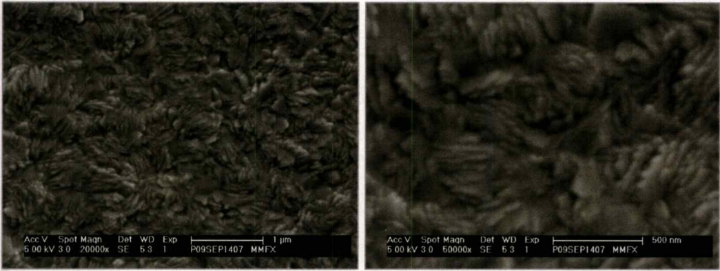
Figure 4.28: Grain of chromium film with substrate bias -160V, SEM image 20,000 X and 50,000X magnification.
