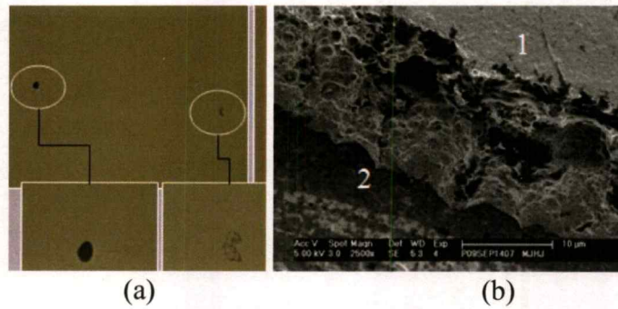
Figure 4.5: (a) Dark spot contamination is taken under high power microscopy. (b) SEM image show approximately 10 μm length. The EDX detail at point 1 show a composition of Cr film. But at point 2 show Cr and C.
