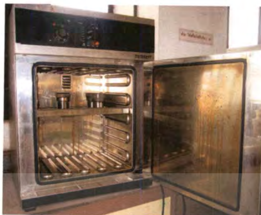
Figure 3.6: Heat Teflon-line autoclave in high temperature oven
