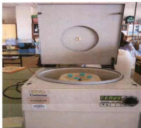
Figure 3.4: Separate catalyst by centrifuge
