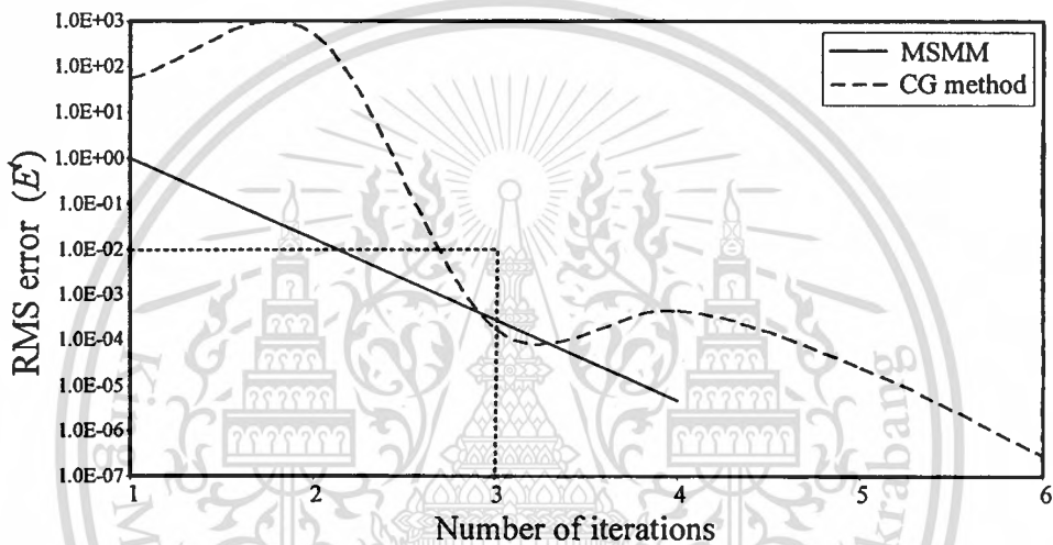
Figure 2.12 RMS errors of the MSMM and the CG method for a uniform collinear dipole antenna array of 100 elements.
