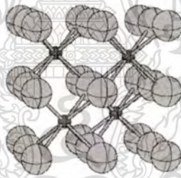
Figure 2.10 Fluorite structure adopted by uraninite ( \text{UO}_2 ) and thorianite ( \text{ThO}_2 ).
