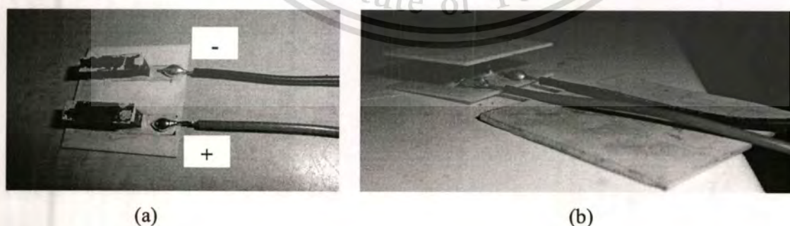
Figure 4.92 (a) The connection of the copper wires, and (b) The topping of the alumina plate.
