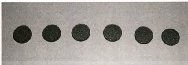
Figure 4.1 The pellets of the CuFeO 2 sinter sample.
