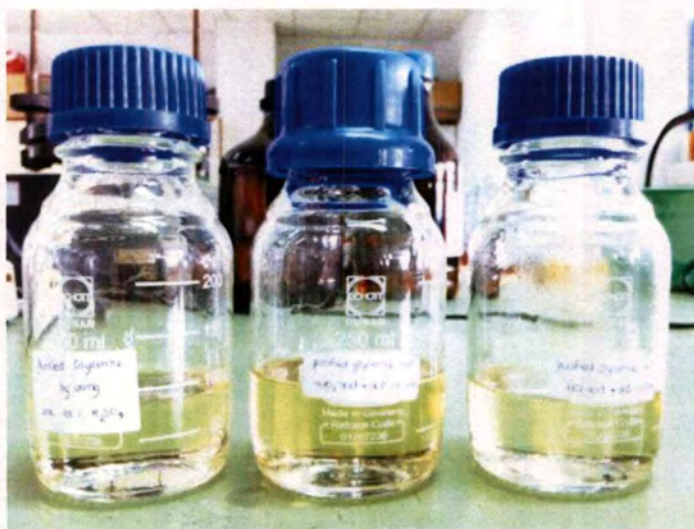
Figure 4.3 Purified glycerol by purification process with sulfuric acid, nitric acid and hydrochloric acid respectively.
