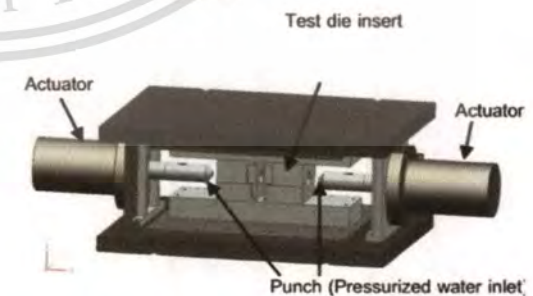
Fig. 12 Schematic diagram of the experimental apparatus for bulge tests
