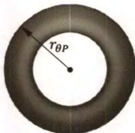
Figure 3.18 r_{\theta P} is circumferential radius of curvature at the pole
