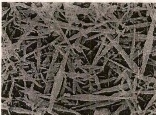
Figure 2.7: SEM image of aragonite (needle-shaped orthorhombic)
