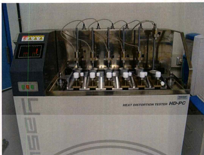
Figure 3.9 HDT/VICAT softening temperature tester (Yasuda model HD-PC)
