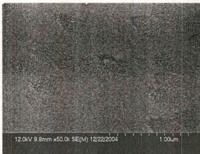
Fig. 6.5 SEM image of 200 nm ITO thin film grown by gas-timing technique.
