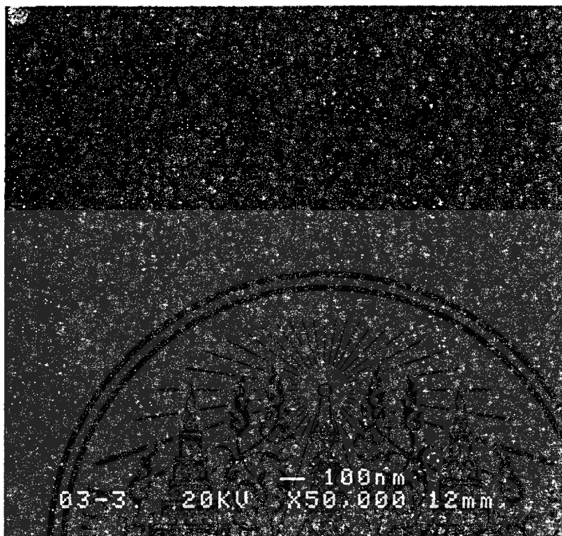
Fig. 7.3 SEM image of 500nm- thick NC-ZnSe film.
