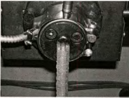
Figure 3.6 The St-Bu-g-starch and PS compounding by single screw extruder.
