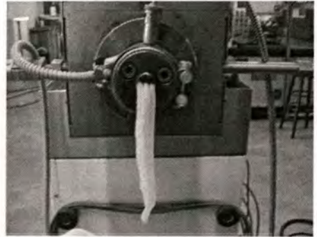
Figure 3.6 The St-Bu-g-starch and PS compounding by single screw extruder.
