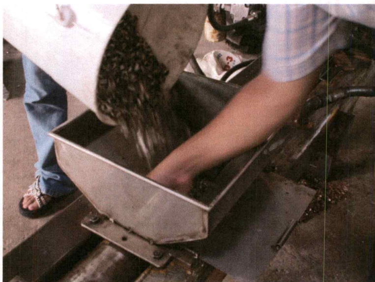
Figure C-8 Pouring the purging nut seeds into the expeller
