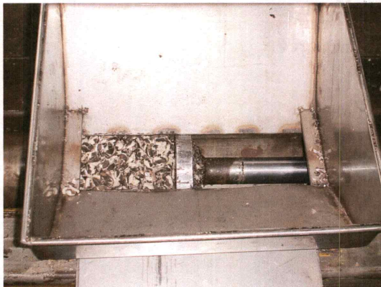
Figure C-9 Pressing the purging nut seeds
