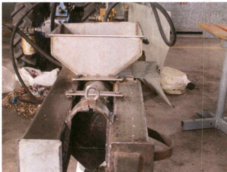
Figure C-7 Expeller for the purging nut seeds
