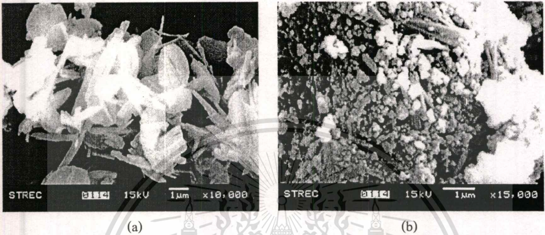
Figure 4.6 Electron micrographs of zeolites encapsulated cobalt phthalocyanine before solvent extraction of (a) Ion-EMT and (b) Ion-BEA
