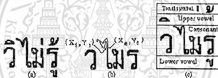
FIGURE 15. Single-character segmentation is base on histogram analysis and contour tracing.
