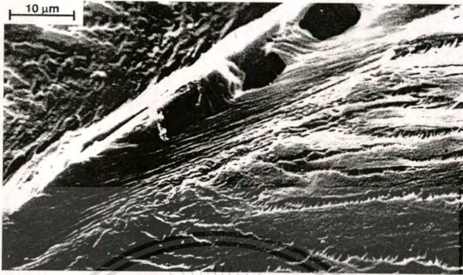
Figure 2.6 Fiber pullout in a rubber-toughness PA-6 composites [8]
