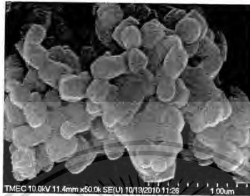
Figure 5. SEM micrographs showing K_{1/2}Na_{1/2}NbO_3 powder obtained from fuel-to-oxidant molar ratio of 0.6.
