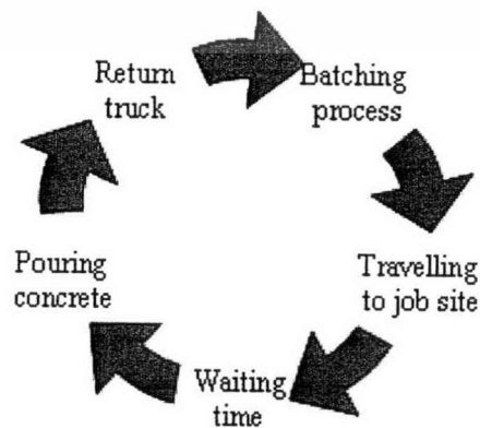
Figure 3.1: Ready mixed concrete delivery process
